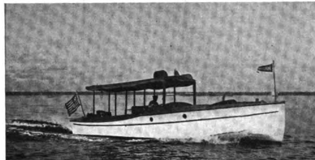
A 30-Ft. Hand V-Bottom Cruiser. Powered with a 40-H.P. Loew-Victor Engine. Speed 15½ M.P.H.
